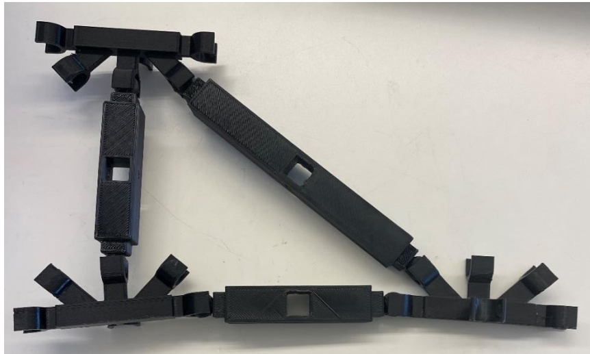
Figure 5. Short and Long members attached to connectors to form triangle.
