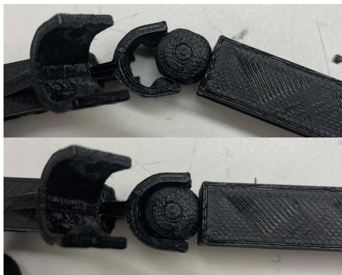
Figure 3. Fitting a bridge member to a connector.
