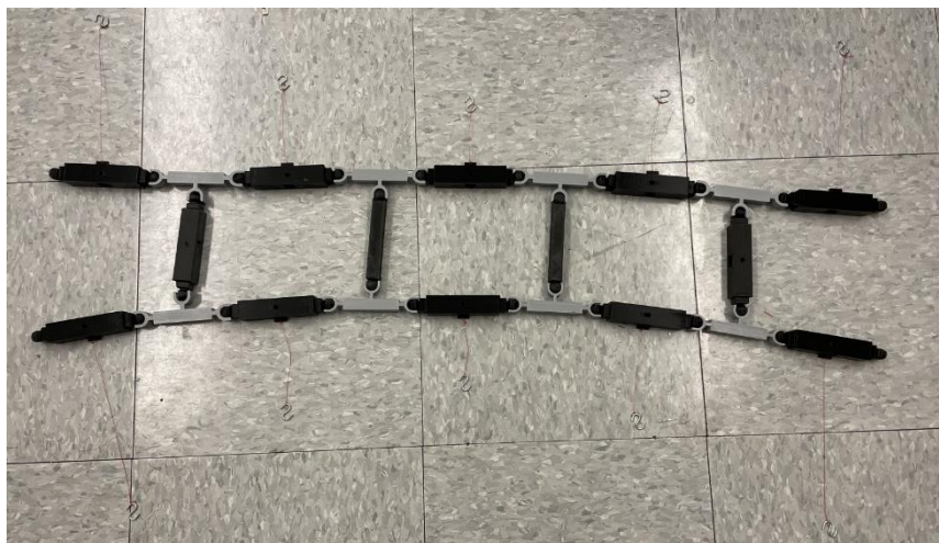
Figure 7. Partially assembled suspension bridge not yet attached to main cable.
