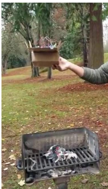
Fig 19: Distance Testing (Smoke Sensor: Directly above flame ~1.5-2ft)
