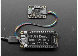
Adafruit HTU31 Temperature & Humidity Sensor Breakout Board -STEMMA QT / Qwiic
